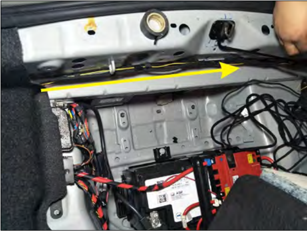
16. Our yellow control cable is routed along the yellow arrow to the control box, fixed the original vehicle harness with the tape.
