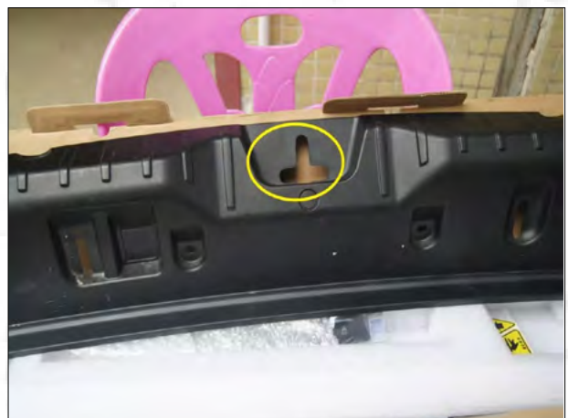
10. Cut a small square slot on the tailgate trim panel.
