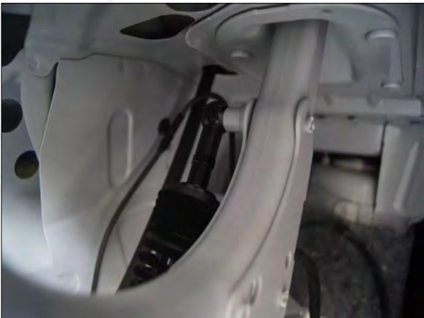
7. As shown in the figure, install the brace rod ( Brace rod toward the body cab ).
