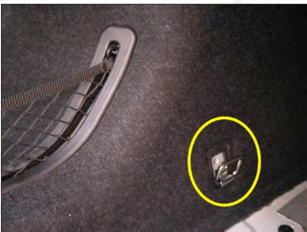
4.Remove the three buckles and remove the left trim panel.
