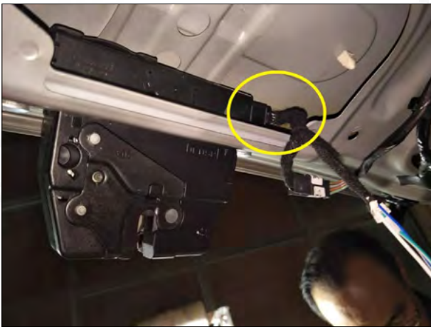
13. Unplug the original vehicle socket at the original door lock and plug our three-way adapter socket. And insert the three-way socket at the other end.
