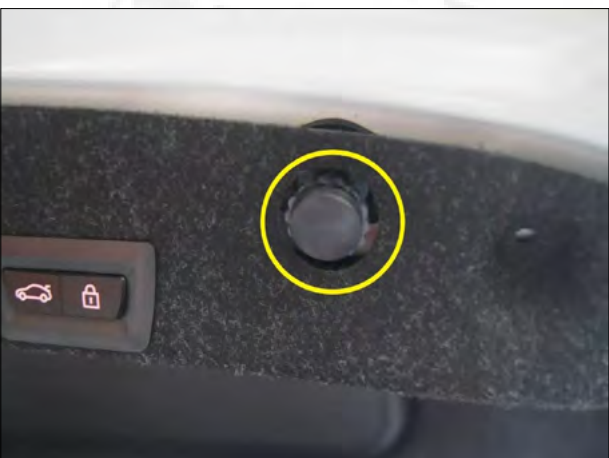
9. Unscrew the screws on the door as shown, and remove the trim panel.
