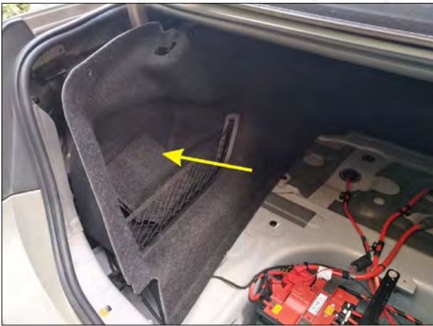
5. Remove the trim panel on the left side of the trunk.
