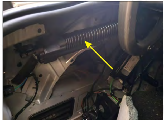
8. Left brace rod installation completed.
