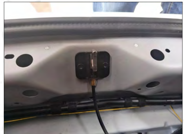
15. Remove the original car lock. Install our electric suction lock and use our screws to fix.
