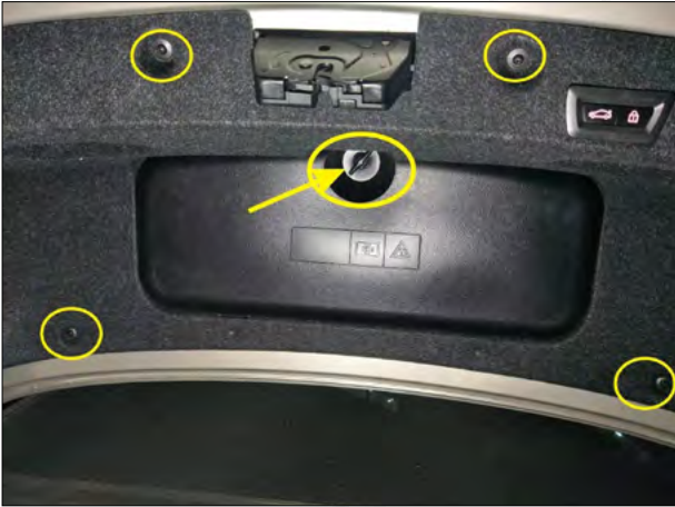
2.Remove the four buckles of the trim panel and remove the trim panel.
