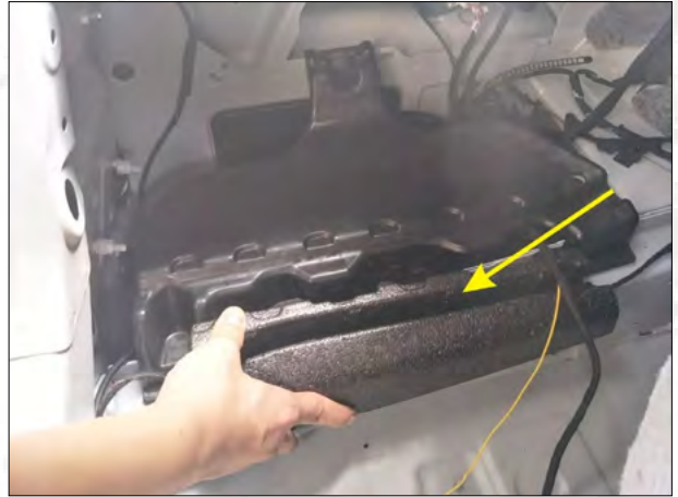
17. Remove the trim panel on the left side of the tailgate and install our control box and motor.
