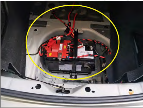
11. The battery can be seen after removing the tailgate cover.
